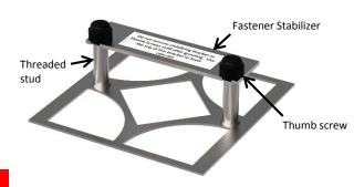
• Each PermaTile<sup>™</sup> Fastener is equipped with a stabilizing bracket. The bracket ensures that basket mounts properly. Remove stabilizer after thin-set has met minimum cure times specified by manufacturer.
